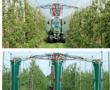
The WIESEL System Flat-Net makes row distances of up to 11 m and clearance heights to a maximum of up to 5 m possible.
