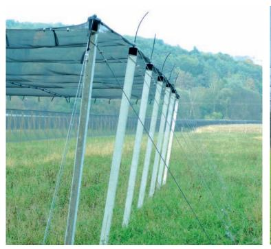
Very sturdy construction by means of tested anchoring in the soil. The WIESEL System Flat-Net is wind and rain permeable and solid at wind speeds of up to 100 km/h (62 mph).
