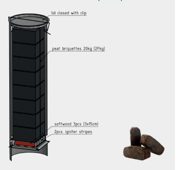
Peat briquettes: foiled in 10 kg packages stacked to the oven specification
