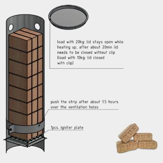
Wood briquettes: foiled in 10 kg packages stacked to the oven specification
