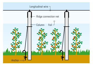
By anchoring the inner column, a very high wind stability is achieved.
